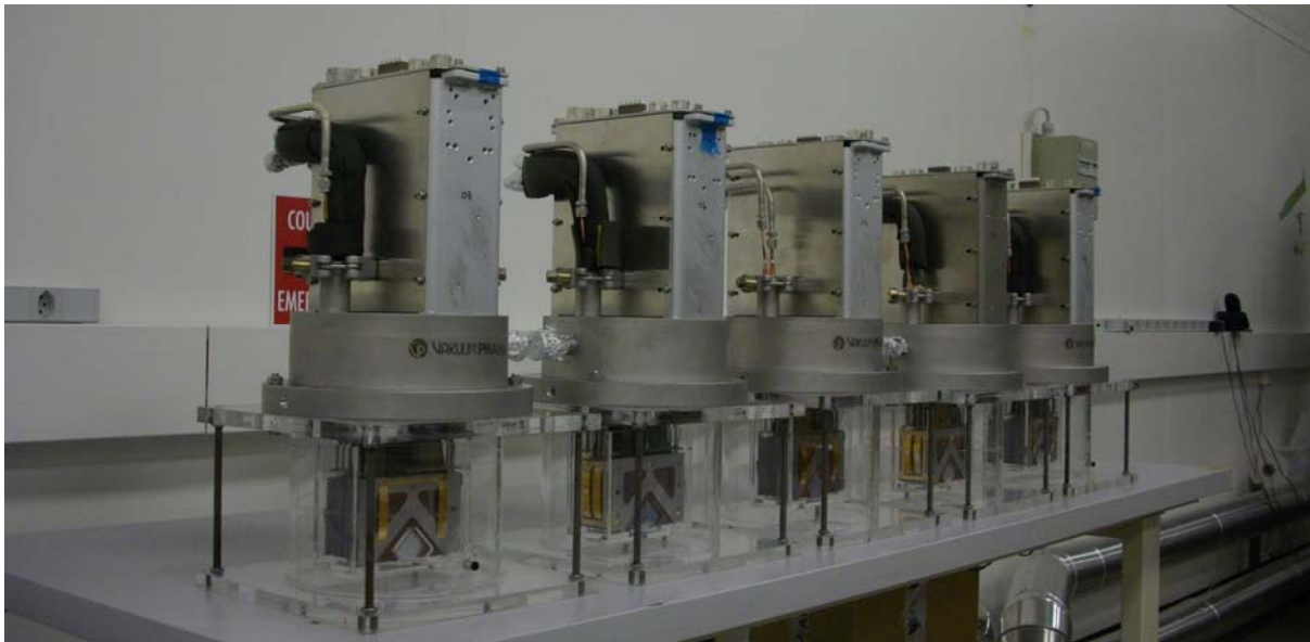
Fig. 3: Five Roman Pot detector assemblies fully tested and ready for installation in the tunnel to complete the station at 220 m in sector 5-6.
