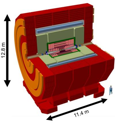
Low-mass all-silicon tracking system with separate tracker and vertex detector
