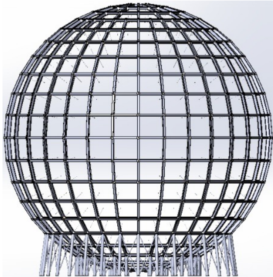
Stainless Steel Truss Inner Diameter: 40.1m
