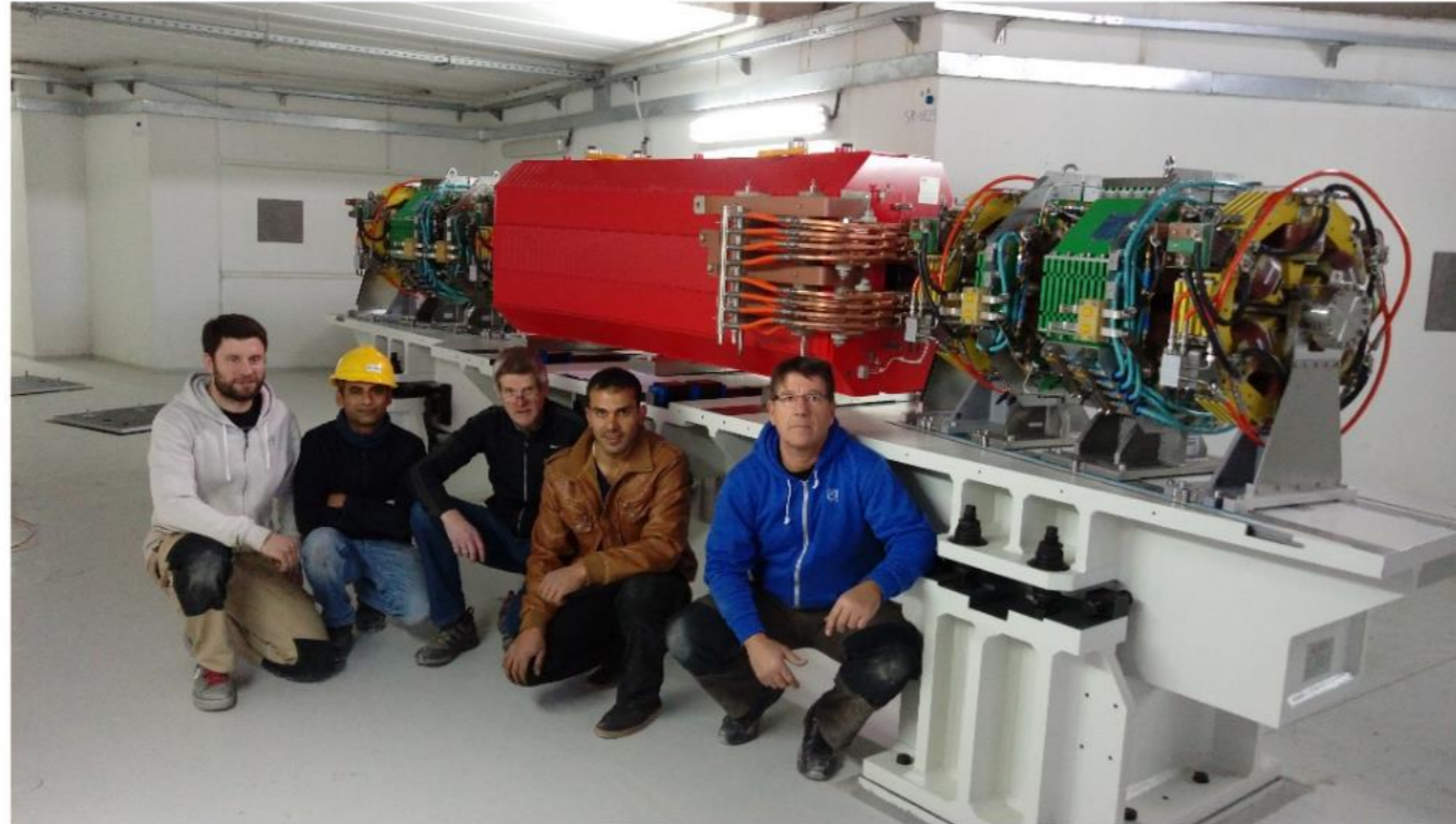
Source of the photo: © SESAME | One cell of the main storage ring installed in the shielding tunnel in the experimental hall with (left to right) Maxime Dumas (CERN), Maher Shehab, Erhard Huttel and Mohamed Khalileh (SESAME) and Carlos Lopez (CERN)
