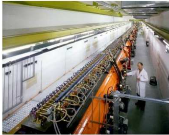
CERN LINAC 2 tank 1: 200 MHz 7 m x 3 tanks, 1 m diameter, final energy 50 MeV.
