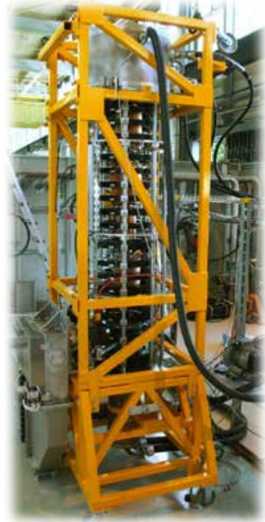
CERN LHC: 400 MHz, 300 kW, CW, \eta 62 %
