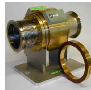
CERN SPS Fast Beam Current Transformer (FBCT)
