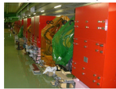
J-PARC collimation system with shielding
