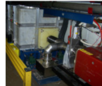
Fermilab collimation system with shielding
