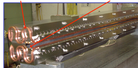
Absorber blocks inspected after impact of HIRADMAT test #6: survived and re-installed
