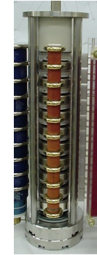
Stack of high-power semiconductor switches (GTOs)
