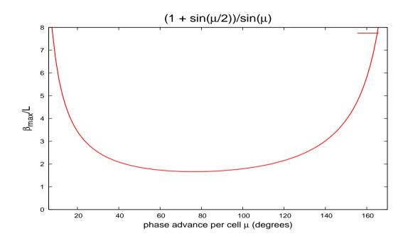
Maximum  $\hat{\beta}/L$  as function of phase advance - should be small enough for aperture
