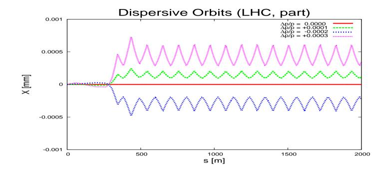
Higher and lower momentum particles on different orbits along part of the LHC ring
