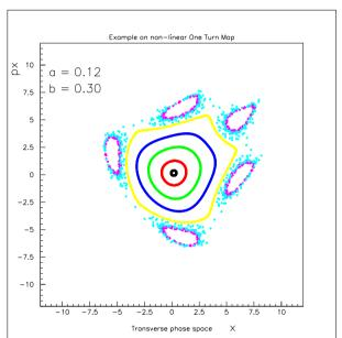
In ideal world: phase space diagrams show ellipses (normalised become <u>circles</u>, was not introduced, but inevitable for beam dynamics calculations)
