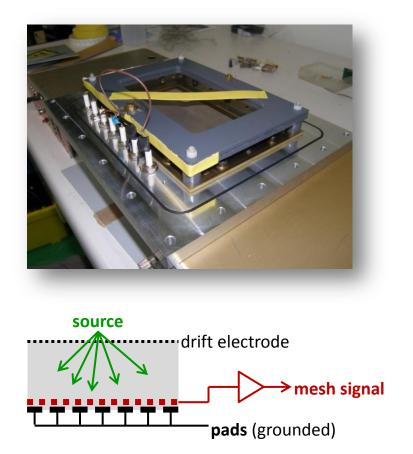
drift volume thickness: **2.5** *cm*  $HV_{mesh} = -570 V$  $HV_{drift} = -1000 V$
