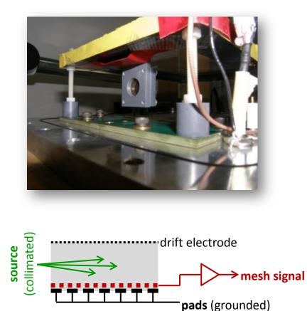
drift volume thickness: **5.0** *cm*  $HV_{mesh} = -370 V$  $HV_{drift} = -1500 V$
