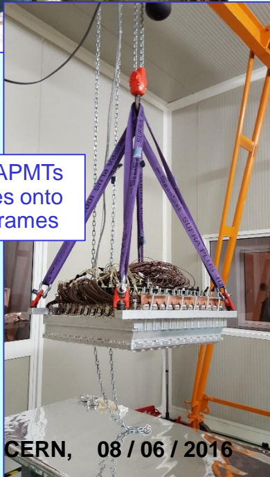
Dismount MAPMTs + lenses from the old detectors
