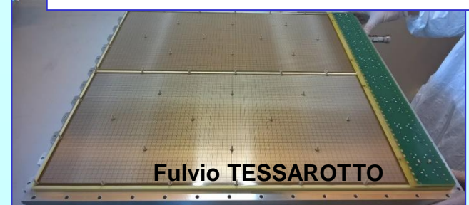
Glueing onto the MM the distance pieces that will ensure the correct distance between MMs and THGEMs
