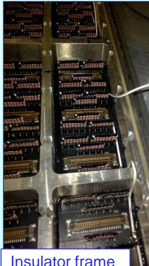
Glueing the insulator frame onto the Al frame that ensures the MM rigidity
