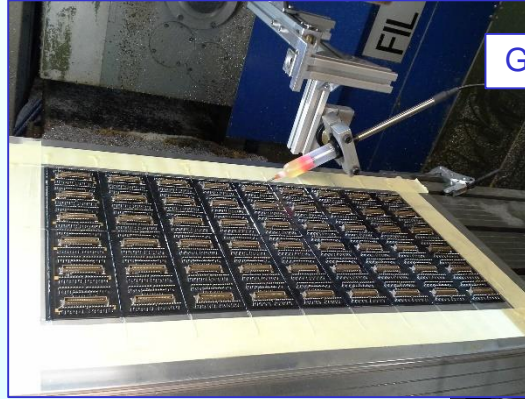
Glueing the insulator frame onto the Al frame that ensures the MM rigidity
