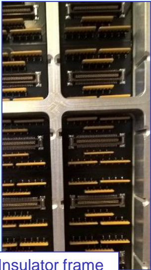
Glueing the insulator frame onto the Al frame that ensures the MM rigidity
