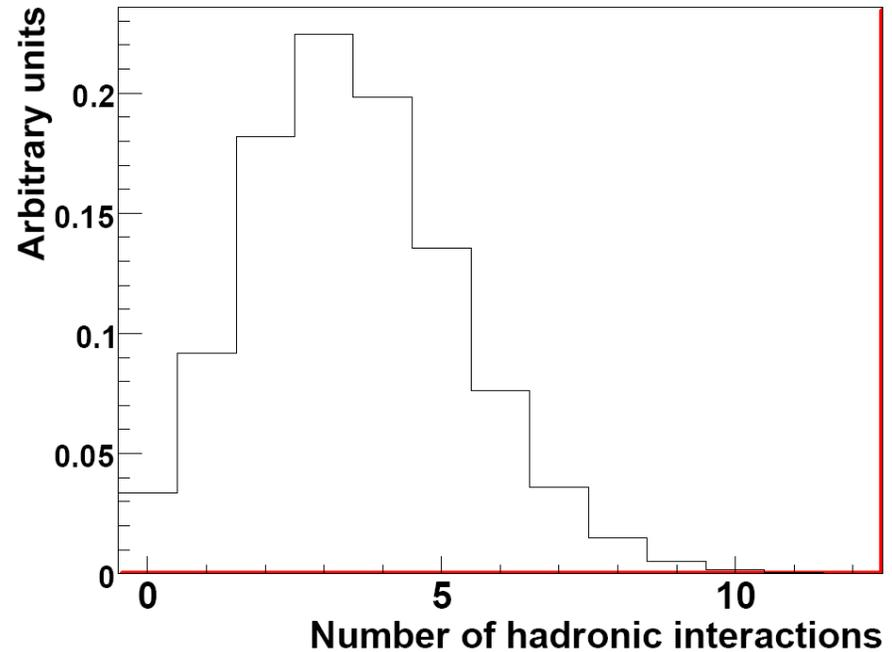
Propagation through 1m of iron with Geant-4 of hadron starting from  $\tilde{g}u\bar{d}$ .
