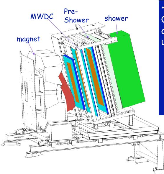
• successfully used for hall A high  $Q^2$  Gen exp.: powerful combination of BigBite + Polarized  $^3$ He target; up to  $L\sim4.5\times10^{36}$  cm $^{-2}$ s $^{-1}$ .
