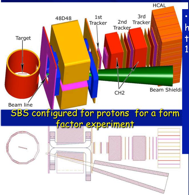
• GEM trackers - much higher luminosity compared to Bigbite; up to  $L\sim 5 \times 10^{38}$  cm<sup>-2</sup>s<sup>-1</sup>.
