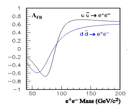
AFB: interference between γ and Z<sup>0</sup> (m<sub>ee</sub>) Different coupling strengths to u and d quarks (compared to leptons) or new gauge bosons change AFB. Use Collins–Soper frame to reduce sensitivity to QCD effects Main uncertainties: **Dominated by statistics**; PDFs, detector resolution Theory becomes relevant for large luminosities (8fb<sup>-1</sup>) Z A<sub>FB</sub>
