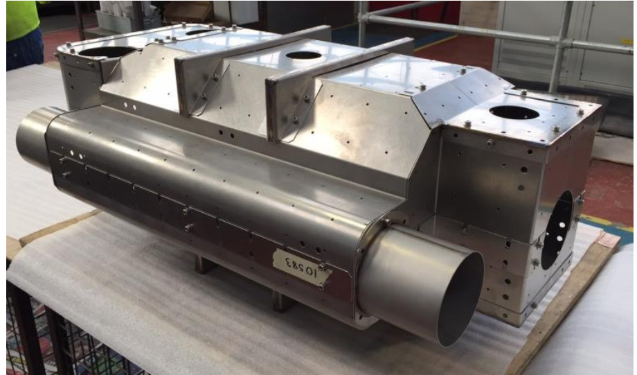
Assembled RFD shield prior to shipping
