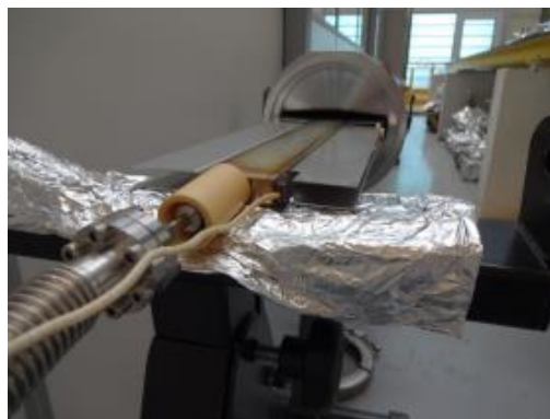
Figure 8: aC coating apparatus for SPS dipole magnets
