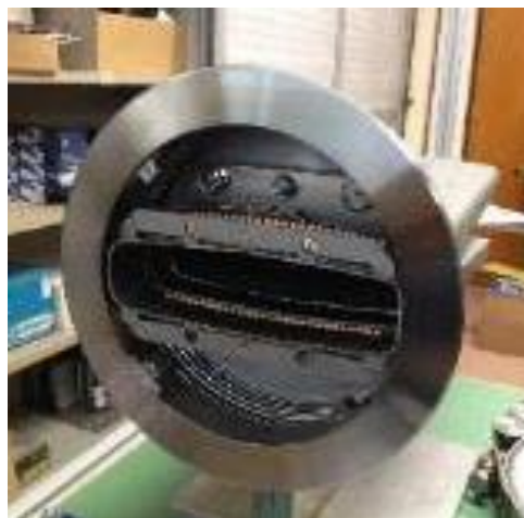
Figure 4: Impedance reduction shielding at SSS QF chamber extremity
