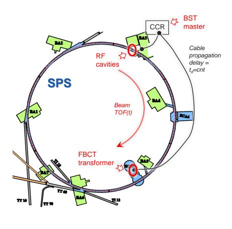
The beam travels from BA3 to BA5 in a certain Time of Flight (TOF) which depends on its energy. TOF from BA3->BA5 ~ 1/3 Trev.
