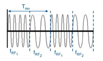
Because ions arrive with too low energy to the SPS, the  $\rm f_{RF}$  signal at the SPS cavities are FSK modulated.
