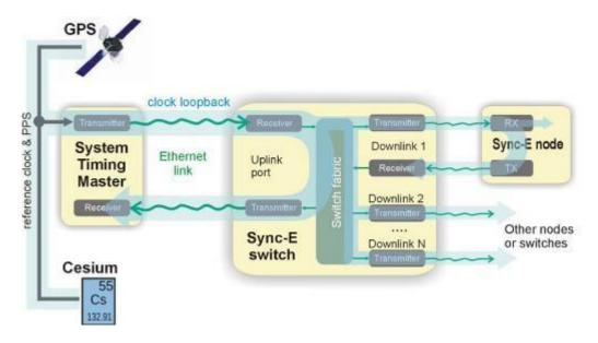
Common clocks allow the use of precise phase measurement techniques (DDMTD) to improve the accuracy of the PTP timestamping and phase tracking.
