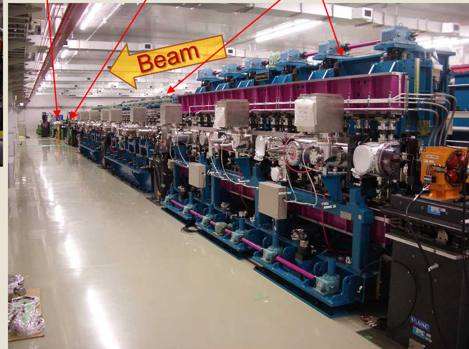
E-gun Buncher cavities BC1 C-band linac BC2
