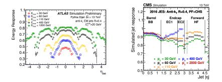
The MC-based calibration accounts for the detector response profile
