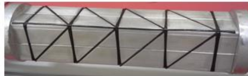
3. Placement of longitudinal reinforcements
