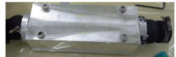
6. Co-curing (internal pressure via inflatable pipe)
