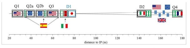
Double layer cos20 Quadrupole Aperture: 90 mm Integrated gradient : 440 T Nominal gradient = 120 T/m 1,9 K Magnetic length : 3.67 m Nominal gradient : 120 T/m Temperature : 1.9 K Nominal current : 4590 A Stored energy : 0.81 MJ
