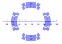
2 layers of MQM cable Inner blocks: 17 + 8 turns Outer blocks: 16 +10 turns
