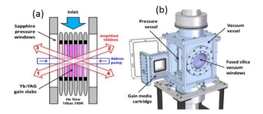
Under development at STFC-RAL (UK) Diode pumped Yb:YAG slabs, He-cooled >100 J output energy demonstrated @ 1 Hz, 1030 nm Ramping up to 10 Hz (design limit): in progress > 60 J conversion @ 515 nm expected
