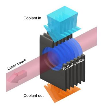
Developed by Dresden Helmoltz Institute Diode-pumped Yb:CaF<sub>2</sub> slabs, He cooled •150 J output energy, •145 fs pulse duration •1 Hz •1030 nm
