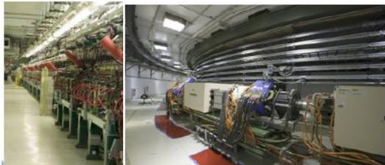
Figure 2-2. a) The 1,000-foot SNS linear accelerator is made up of three different types of accelerators. It is the first of its kind used to generate a pulsed energy beam. b) The SNS ring intensifies the high-speed ion beam and shoots it at the mercury target 60 times a second (60 Hz).
