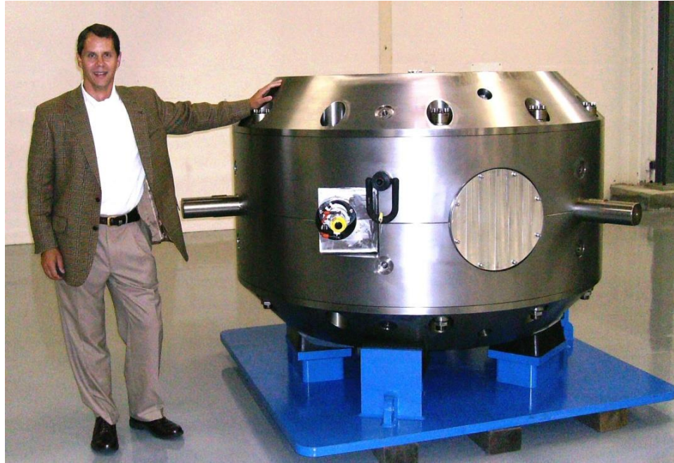
Founder Ken Gall with the MEVION S250 Cyclotron - 17 tons , 8.5 Tesla, 250 MeV
