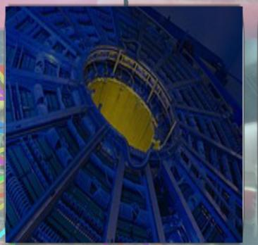
The ALICE Time Projection Chamber (TPC) is a large volume filled with a gaseous detection medium and is the primary particle tracking device in ALICE. As charged particles move through the
