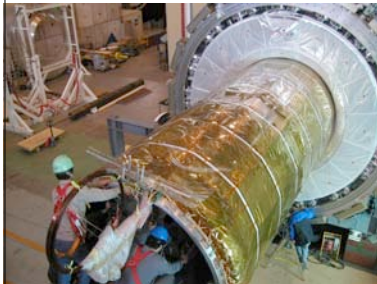
Inserted in the LAr cryostat and fully tested on surface in 2004
