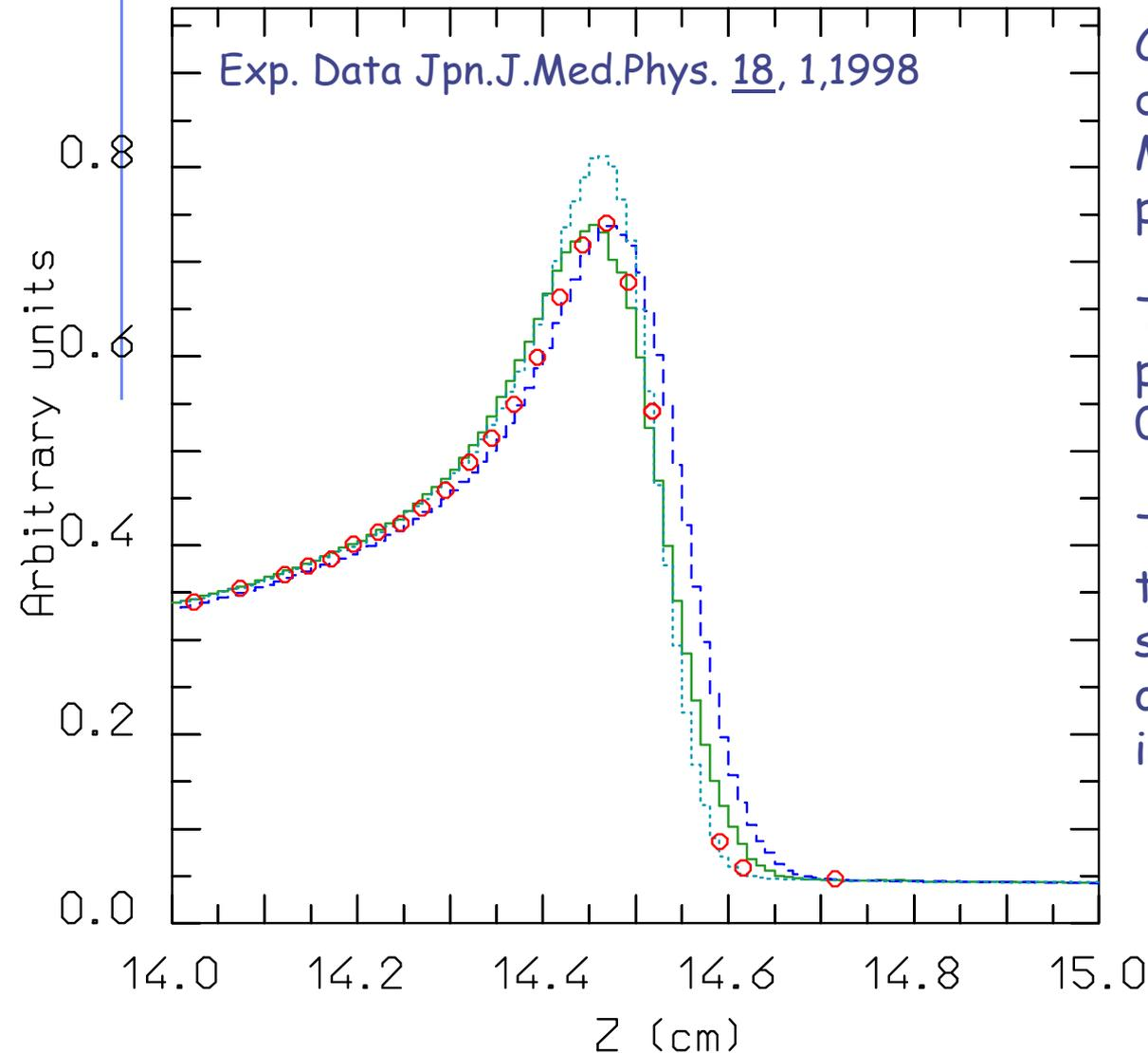
Close-up of the dose vs depth distribution for 270 MeV/n  $^{12}\text{C}$  ions on a water phantom.
