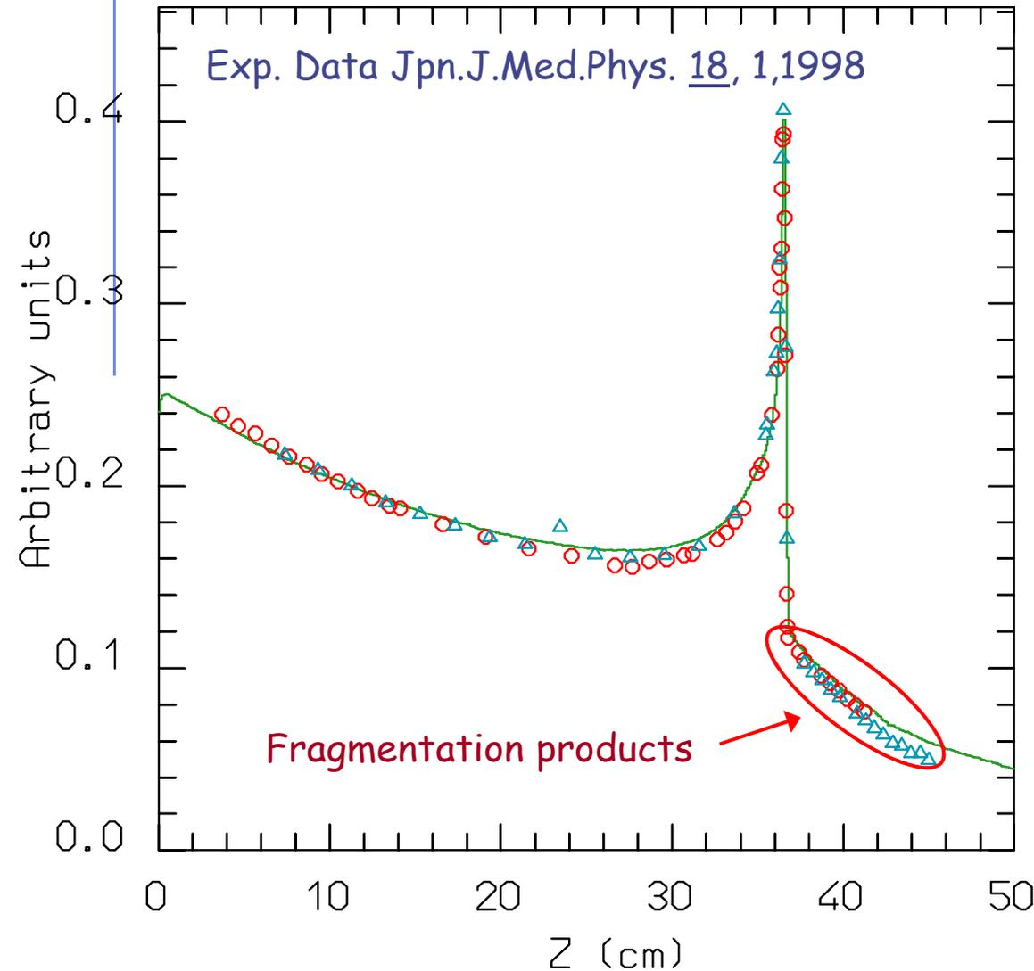
Dose vs depth distribution for 670 MeV/n  $^{20}\text{Ne}$  ions on a water phantom.
