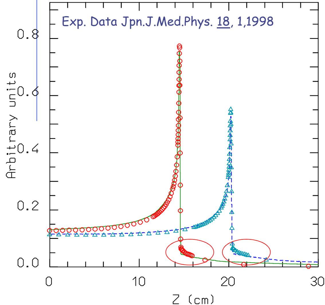
Dose vs depth distribution for 270 and 330 MeV/n  $^{12}\text{C}$  ions on a water phantom.
