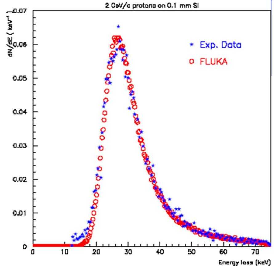
Experimental<sup>1</sup> and calculated energy loss distributions for 2 GeV/c positrons (left) and protons (right) traversing 100 $\mu\text{m}$  of Si
