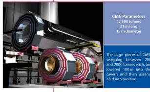
CMS Parameters 12 500 tonnes 21 m long 15 m diameter
