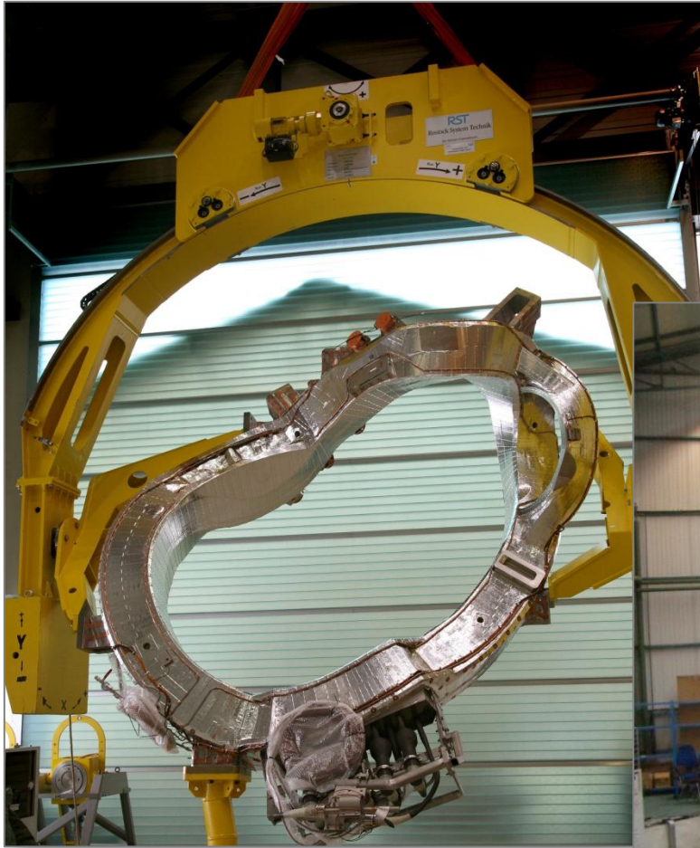
coil in the assembly handling unit
