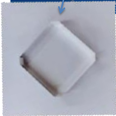
\text{CeF}_3 plate 24*24*10\text{mm}^3
