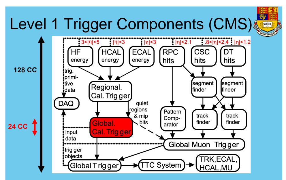
Level-1 Decision is based on Calorimeter and Muon information (as in ATLAS also)
