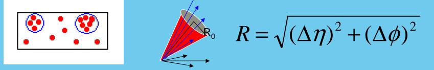
• Energy depositions within a cone are combined and the Et weighted  $\eta$  is calculated:
