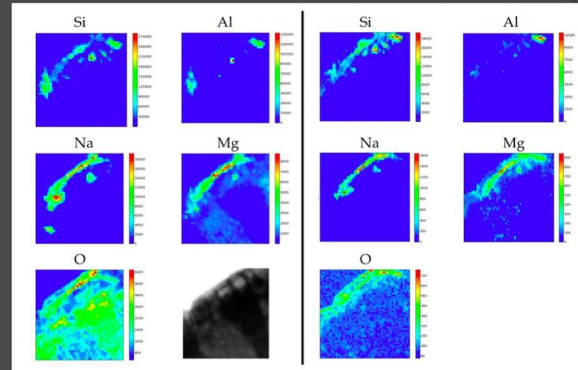
Si-Al-Mg-Na-O spectra of a *euphorbia pityusa* plant section acquired with one cell of the new TwinMic detector and with 6 SDDs of the standard system
