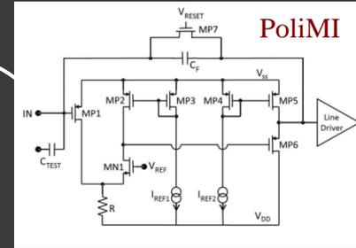
Low-power and very-low noise optimized preampl. in sub-micron technology **PoliMI**
