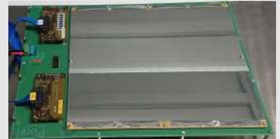
Detector with HV foils end electronic boards
