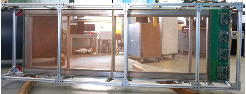
2.8m x 1.0m, 1024 sensing wires
