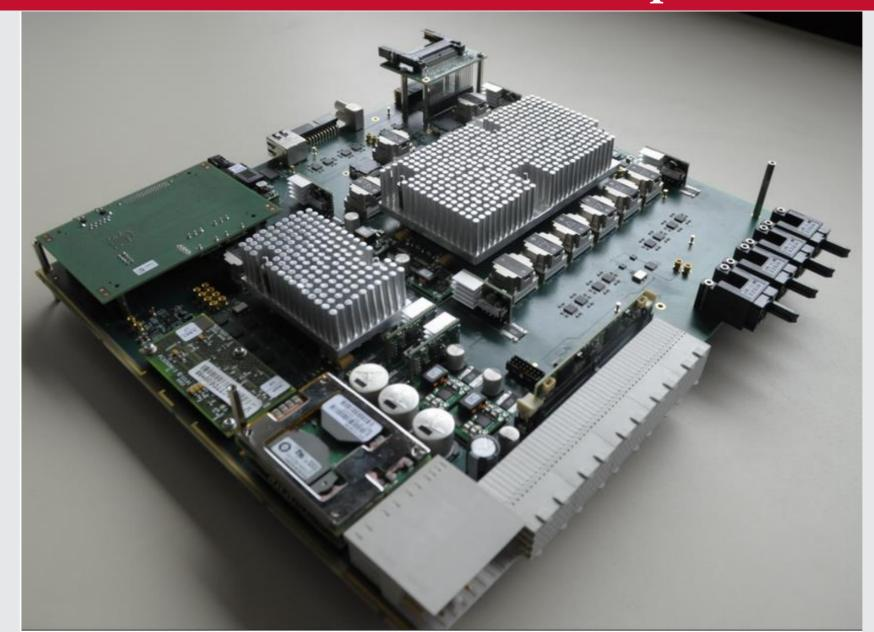
L1Topo processes about  $1 \, \text{Tbit s}^{-1}$  of input data with a fixed latency of  $\sim 200 \, \text{ns}$ . The input data are received via optical fibres, transformed into electrical signals and then directed into the processor FPGAs (Xilinx Virtex7) where the topological algorithms are applied.
