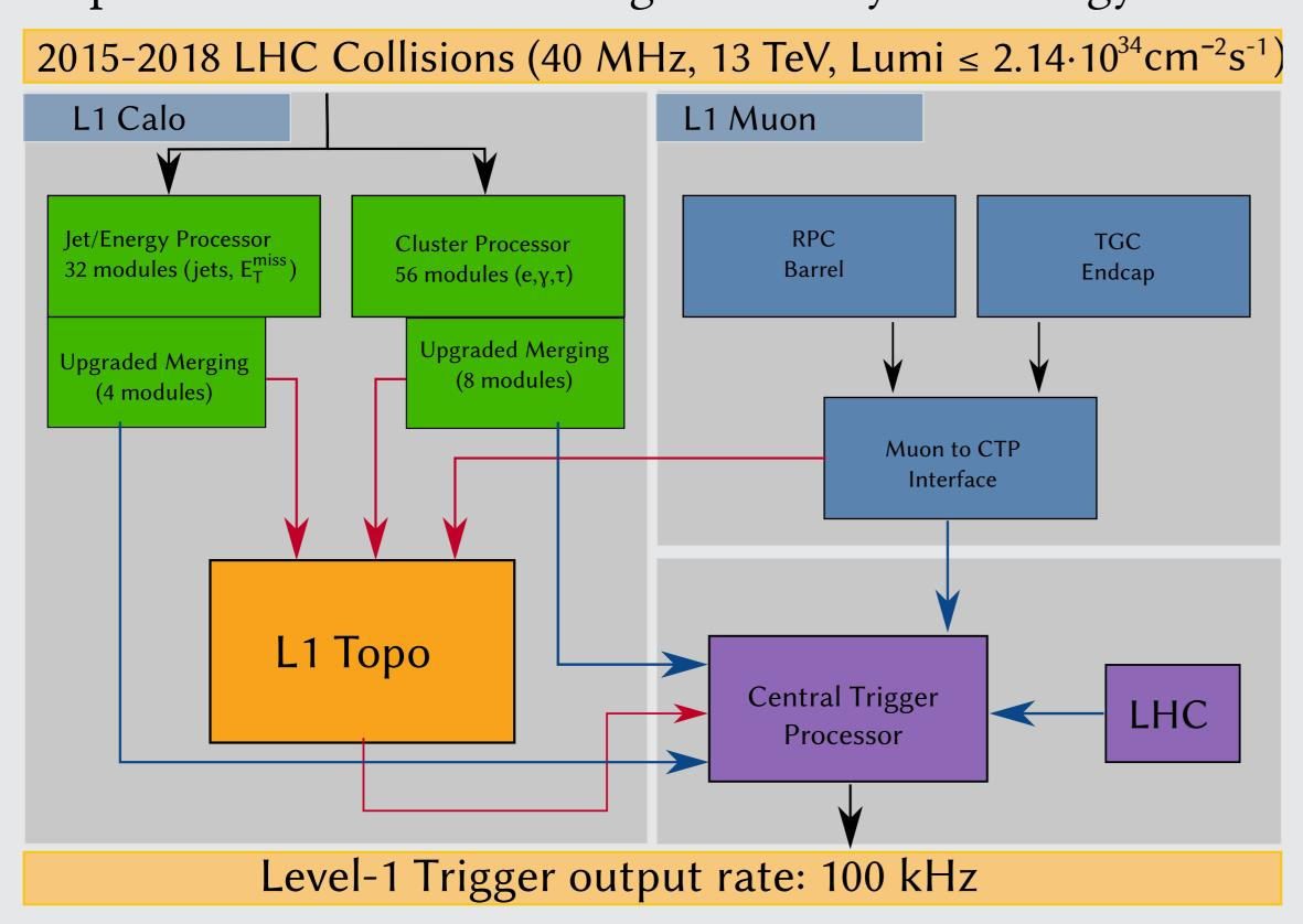
L1Topo gets inputs from the Level-1 Calorimeter Trigger and the Level-1 Muon Trigger containing information on jets, e,  $\gamma$ ,  $\tau$  and missing energy. Its purpose is to provide trigger decisions based on topological algorithms already on the first trigger level.
