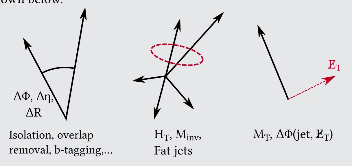
L1Topo triggers are used for different purposes, both for physics as well as for detector calibrations. Various examples with their physics use cases are listed below.
