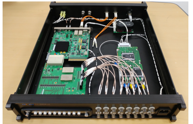
Fig. 2. Manufactured MicroTCA.4 based remote DAQ.
