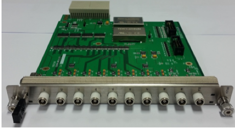
Fig. 4. Manufactured \mu RTM board.
