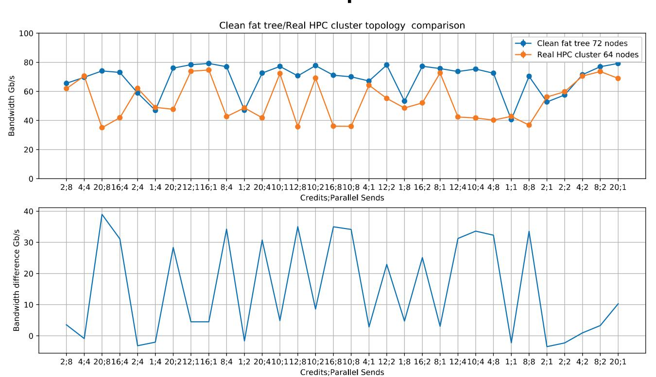
This plot shows the comparison between two runs of the OMNeT++ simulated DAQPIPE with different Infiniband EDR based network topologies: a fat-tree of 72 nodes and imperfect fat-tree of 64 nodes.
