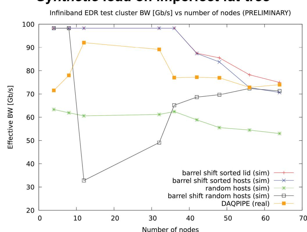
This plot shows the comparison between an ideal barrel shifter simulated with OMNeT++ and a real DAQPIPE run, in both cases the topology is an imperfect fat-tree of 64 Infiniband EDR nodes.
