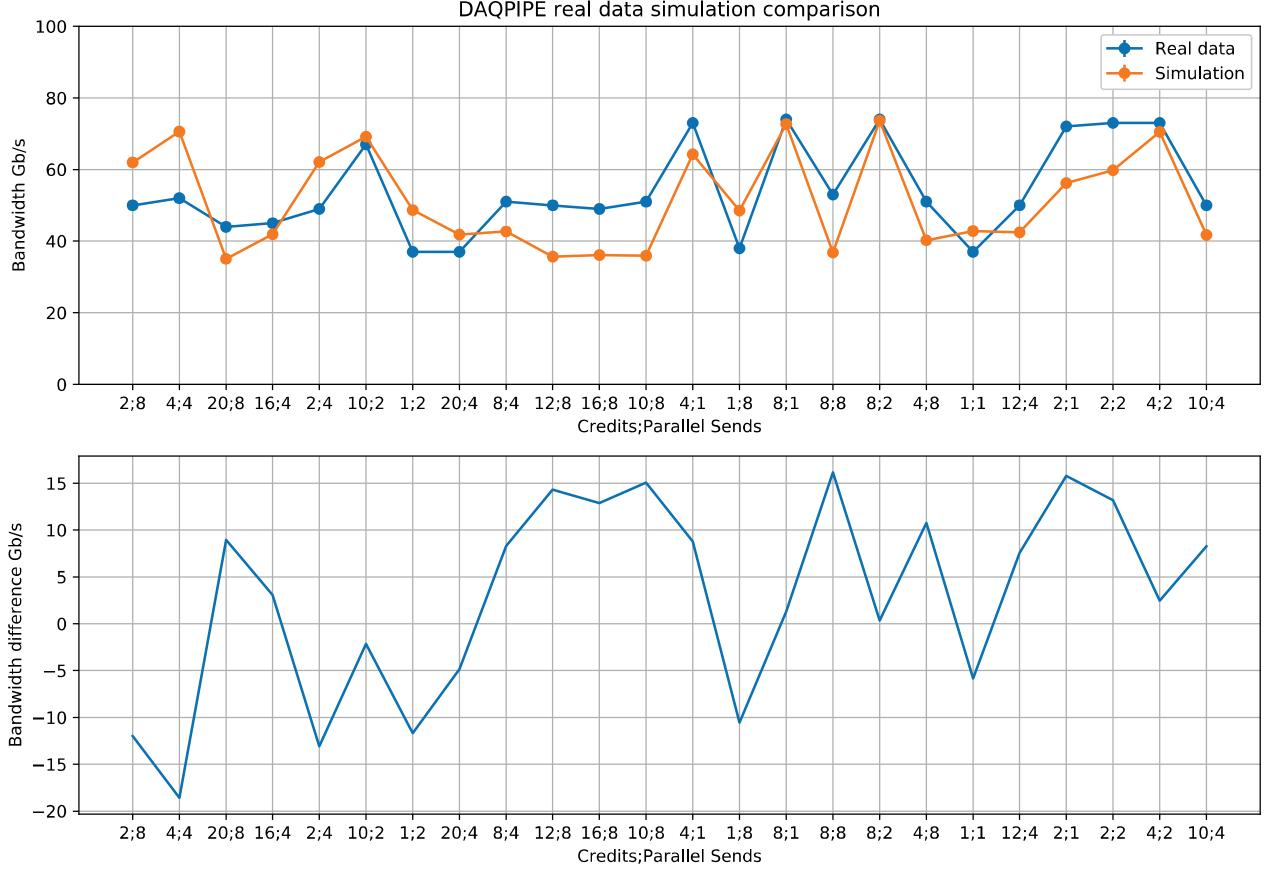
This plot shows the comparison between a real DAQPIPE run and a simulated one using OMNeT++, for different parameters. In both cases the underlying network topology is an imperfect fat-tree of 64 nodes interconnected by Infiniband EDR (100 Gb/s).
