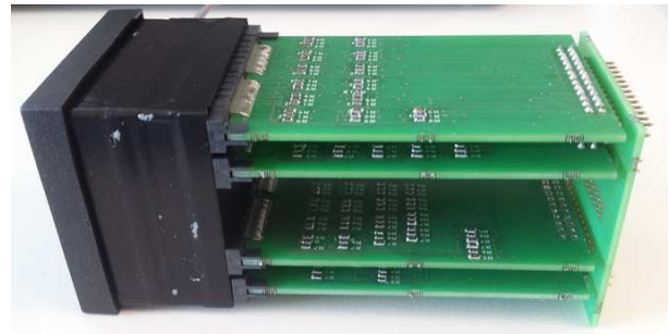
Fig. 3. A network of 507 resistors that reduces the number of output signals from 169 to 26 (13 on X and 13 in Y axis).
