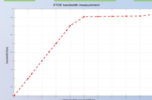
The source from 0 to 10Gbps are generated via two clock (125MHz 156.25mhz) and different bit width data. At the same time ,IPERF measure the bandwidth as the server port.
