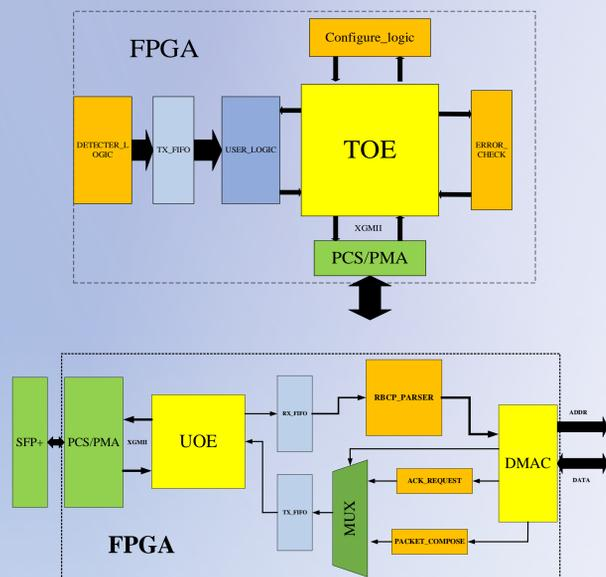
Simple block diagram of the FPGA firmware.
