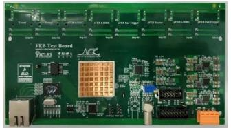
Fig.4. Photograph of the front-end board
