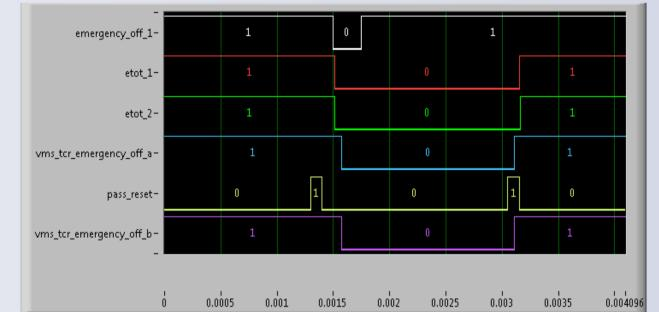
In order to guarantee the correct behavior of the test stand and to be able to trust the unit testing reports, it was calibrated. We chose subset of real unit tests which were manipulated in a way that the test stand application should detect errors at an expected time.
