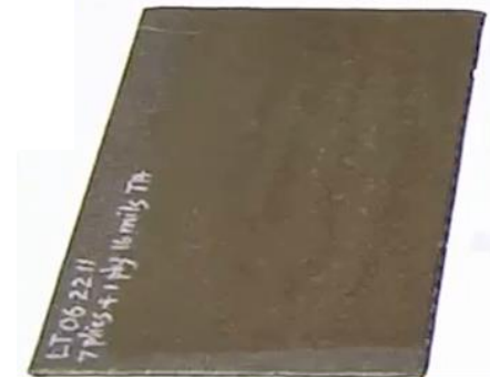
LaRC Ta Carbon Fiber Laminate, prepared by Vacuum Assisted Resin Transfer Molding (VARTM)
