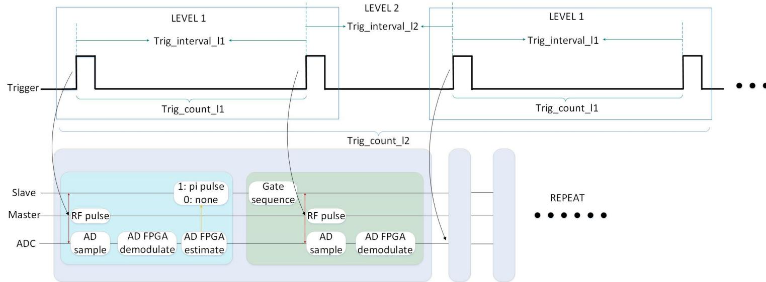
Fig 3. The Timing Diagram of Trigger Mechanism
