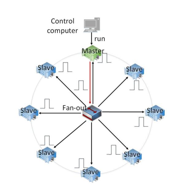
Fig 4. The Star-like Fanning Out Structure
