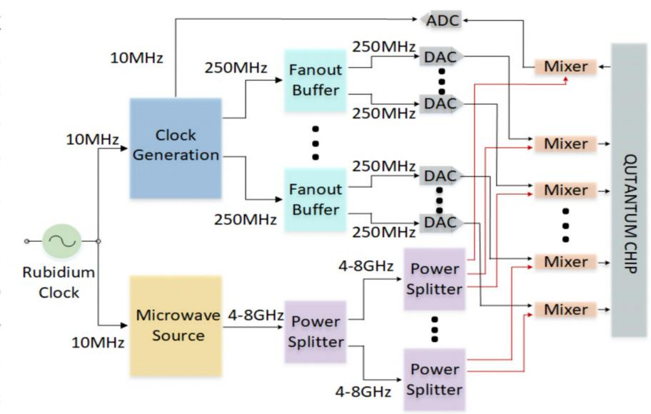
Fig 2. The Structure of Clock Tree
