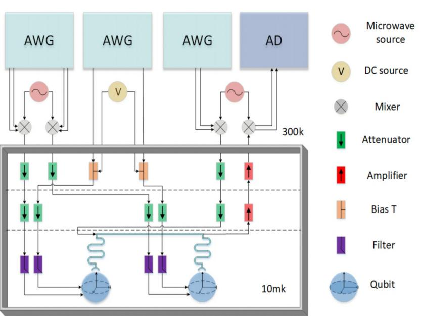
Fig 1. The Experiment Equipment of SQC
