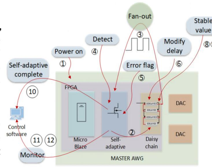
Fig 5. The Process of Self-adaption
