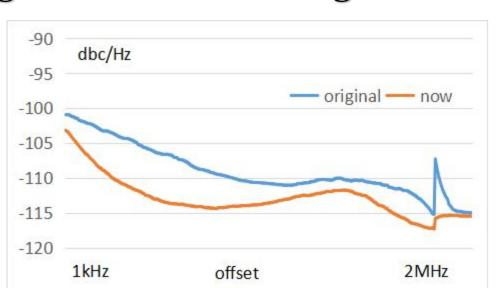
Fig 6.a Phase Noise Comparision of DAC Output
