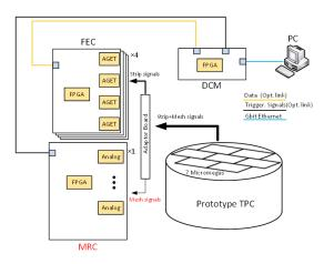
MRC acquire all mesh signals and generates individual 'Mesh-trigger' signals
