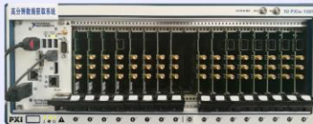
Fig.1: A photo of the PXI-based, Multi-channel Ultra-fast DAS for Transient Pulsed Signal. (Note: The NI PXIe-1085 16-slot chassis features a high-bandwidth, all-hybrid backplane to meet a wide range of high-performance test.)
