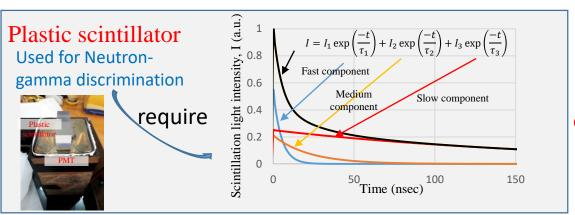
Neutron/gamma discrimination detector by PSD technique
