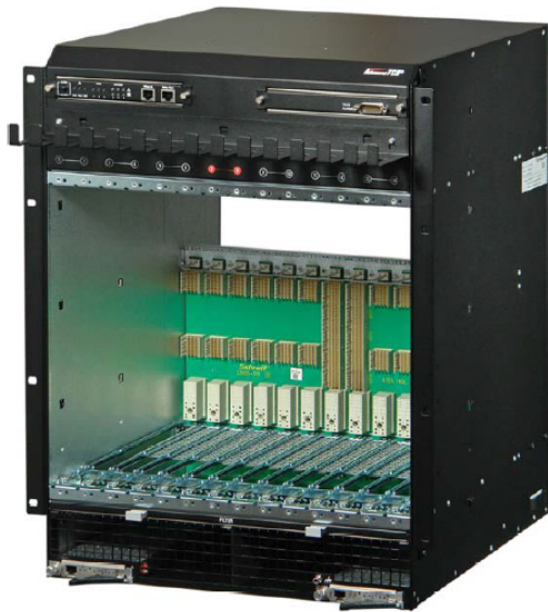
14U 14 Slot Front-to-rear cooling 300W/slot
