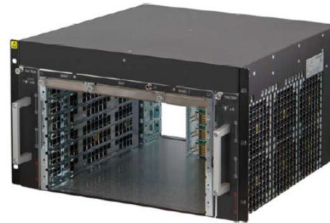
6U 6 Slots Right-to-left cooling 450W/slot
