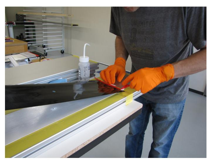
**Optical-quality cuts** are made on both ends of the mat. A diamond milling tool is used in order to maximize the light transmission through the cut surface.
