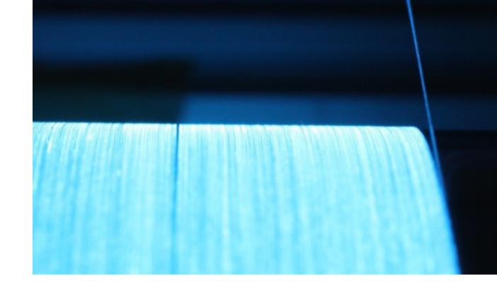
**Casting**: After the winding and the glue curing, the fibre mat is taken off the wheel. A 25- $\mu$ m kapton foil is glued on both sides for optical and mechanical protection.
