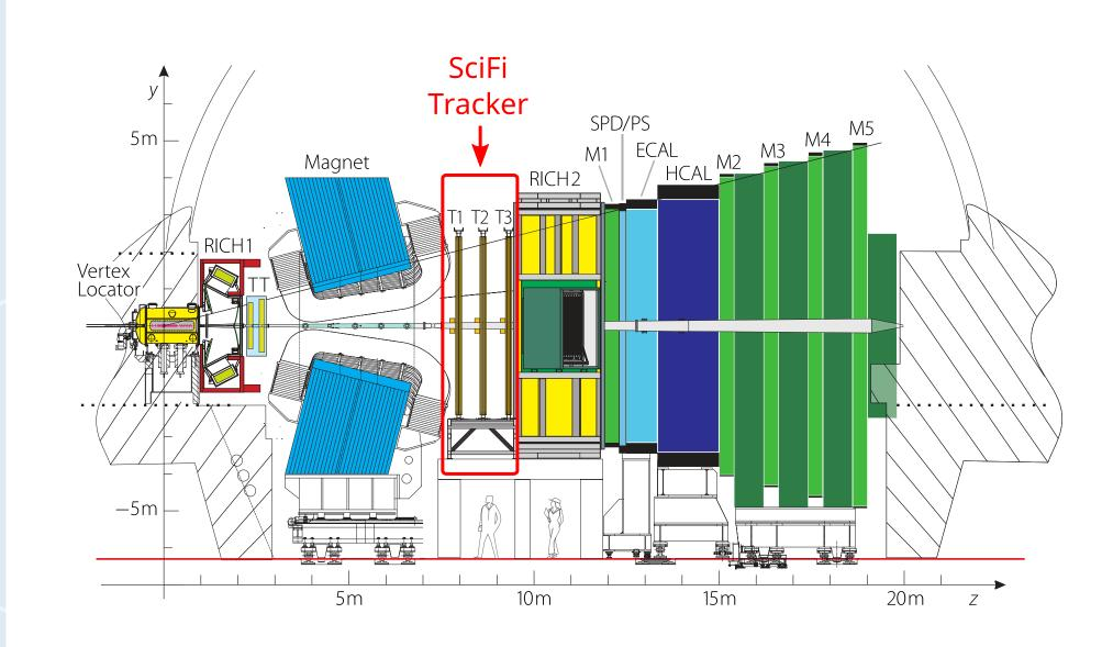
One of the major improvements is the addition of a new scintillating fibre tracker. It will replace the current tracking stations which use straw-tube and silicon-strip technology. The scintillation light will propagate along the fibres and will be detected by silicon photomultipliers (SiPM) at the top and at the bottom of the detector. Mirrors will be used at the middle of the detector to increase the detected signal.
