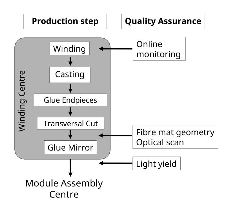
Winding: A winding machine, specifically developed for the SciFi project, is used to lay 6 layers of fibre and glue onto a threaded wheel. PLC-based system provides accurate and realiable control over the speed, tension and the position of the fibre. A video camera and a laser
