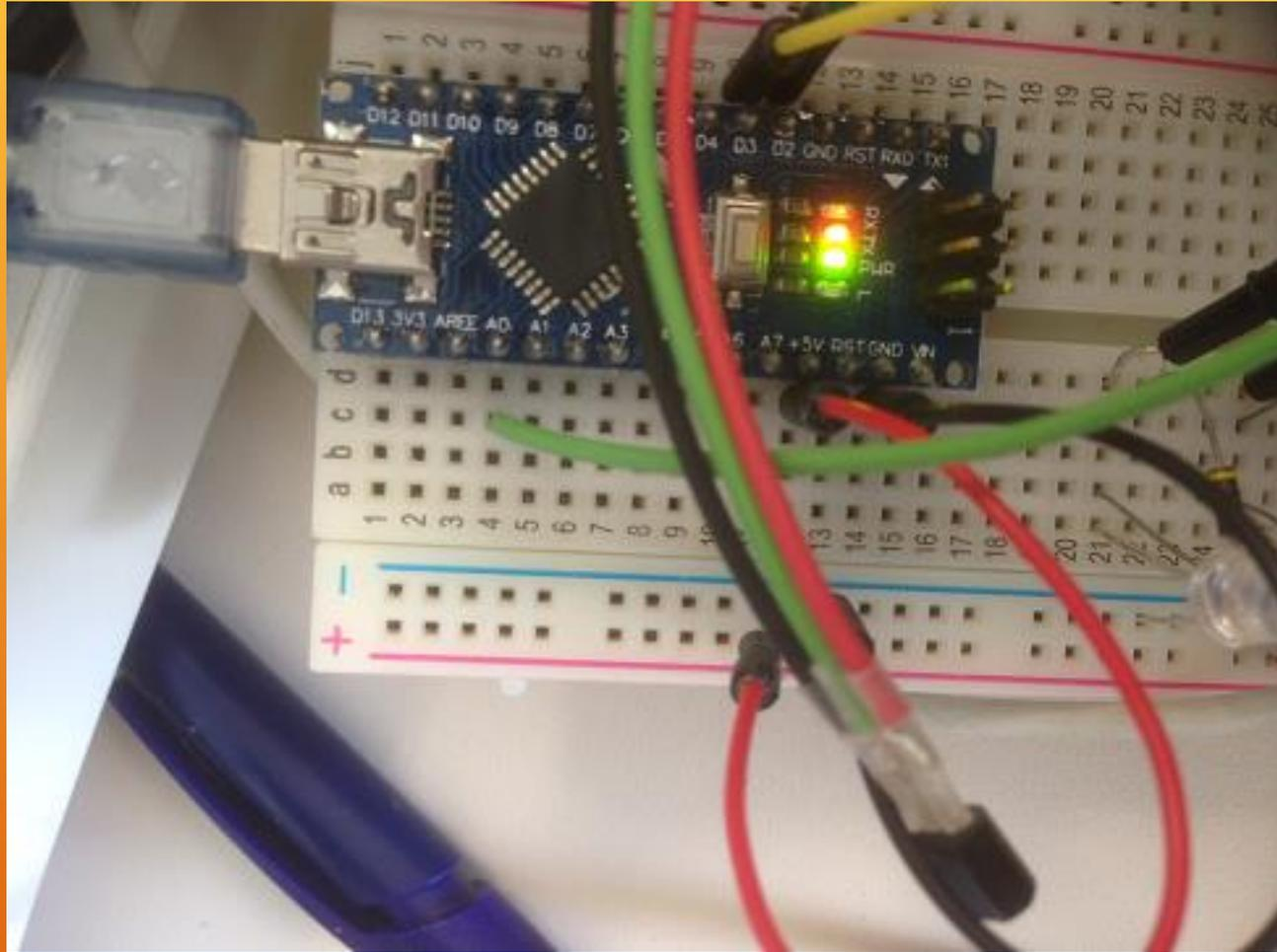
**Analog sensor connections ; powering and A0 as readout channel for a temperature sensor LM35DZ (+150 to 0°C, or other)**
